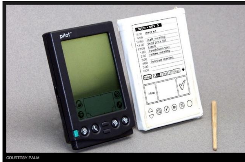
Figure 6: Mockup of the Palm Pilot made of wood and paper 17
